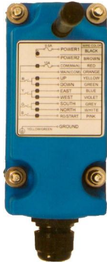
TM2200HT Receiver (AC and DC alike) Contact Control Chief for correct replacement.
